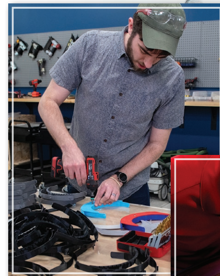
Instructional technician Max Wheeler assembles face shields with parts manufactured at Innovation Studio.
