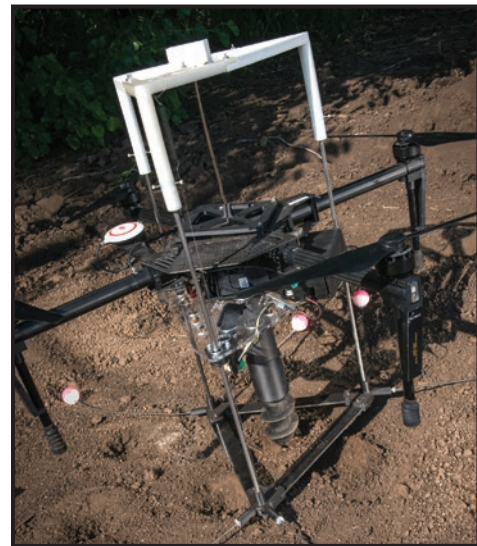
Drone with drill probe attached
